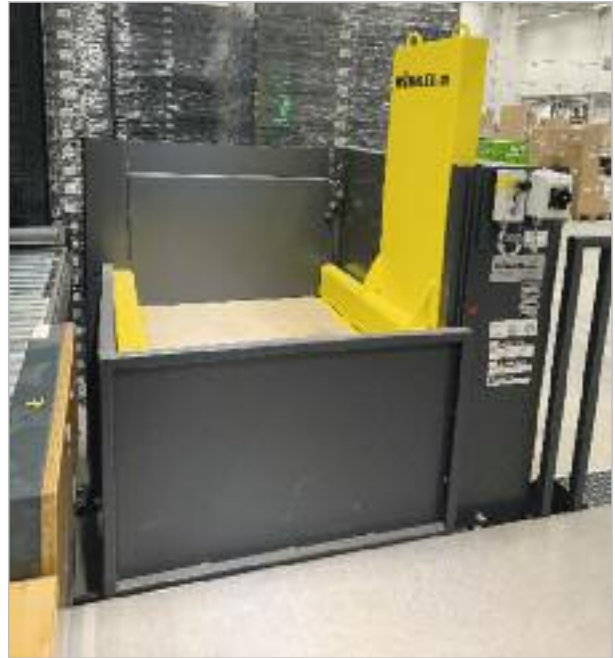
Pallet station for roller cages and pallets
