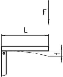
$$f [\text{mm}] = \frac{0.476 \times F [\text{N}] \times L^3 [\text{m}]}{I [\text{cm}^4]}$$
