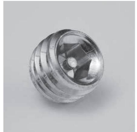
Special PVS® screw Safe M12x12 for safety constructions which must not be easy to dismantle by unauthorised persons. A pin inhibits access to the screw so that it cannot be unscrewed using a commercially available Allen key.
