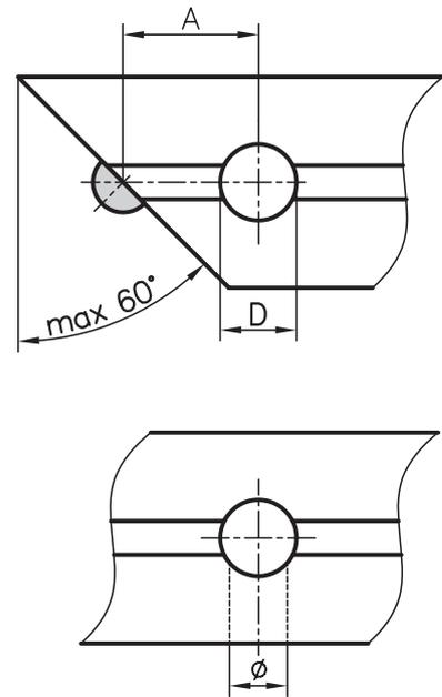
That drill, allows a connection for a parallel connector at any position at the extrusion.
