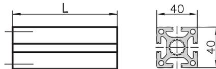
2c. Cutting the extrusions to length and threads according to drawing
