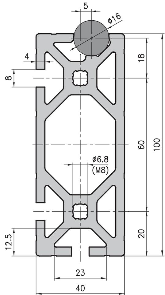
the front face in the holes  $\text{Ø} 6.8$  with a M8 thread.
