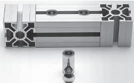
The round anchor head allows the extrusions to be set in any position, however it must first be pushed into the retaining slot. **Also available in stainless steel or providing electrical bonding. (electrically conducting)**
