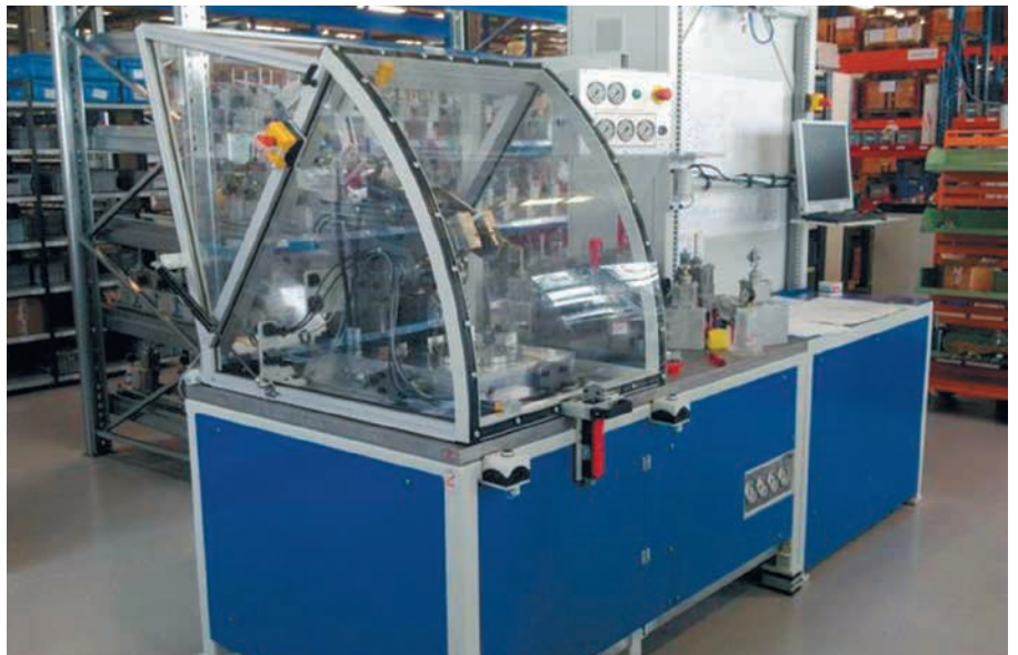
Pneumatic swing lift doors
