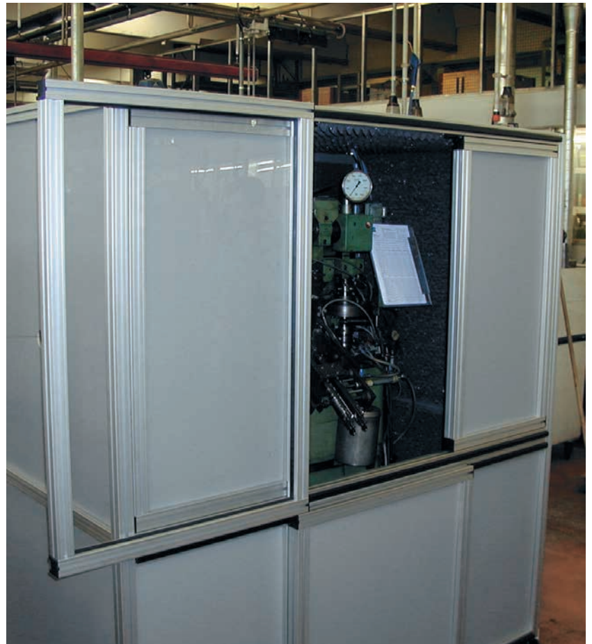
Acoustic protection cabin
