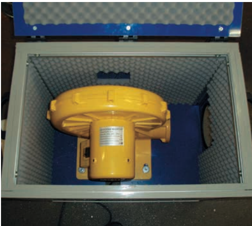
Acoustic protection box for blower
