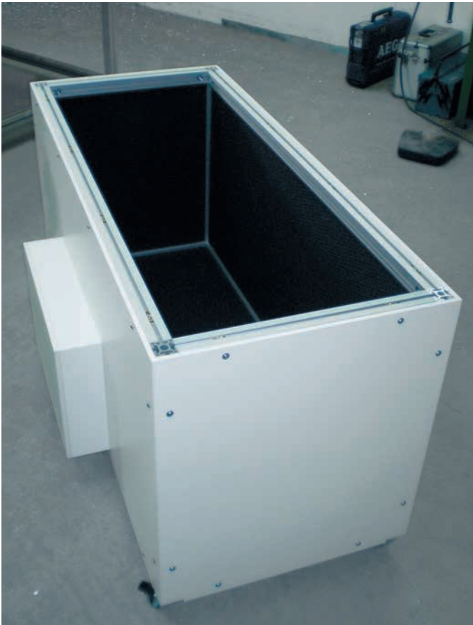
Mobile noise protection housing with ventilation system for a vacuum pump
