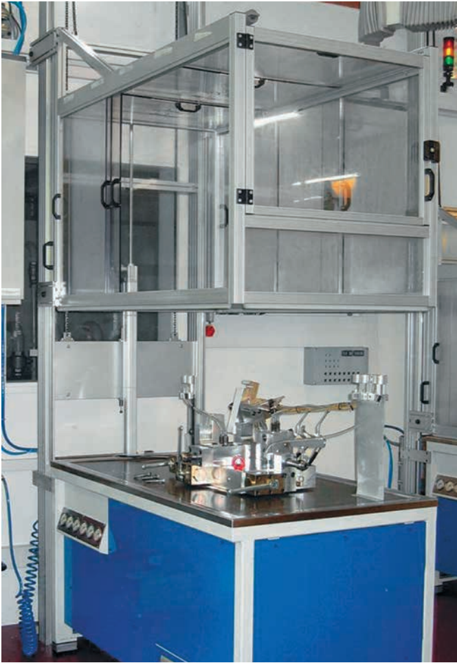
Protective hood with counterweight
