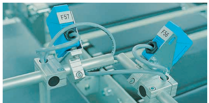
An easily adjustable photocell fixture.
