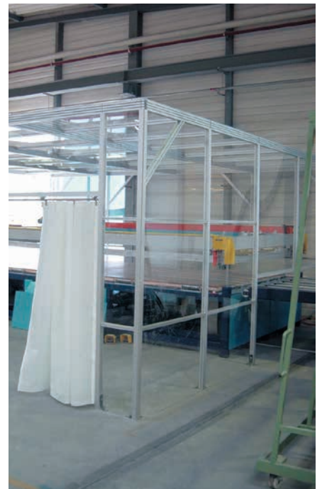
Dust protection cabin
