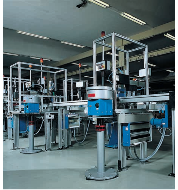
Feeder and transfer system
