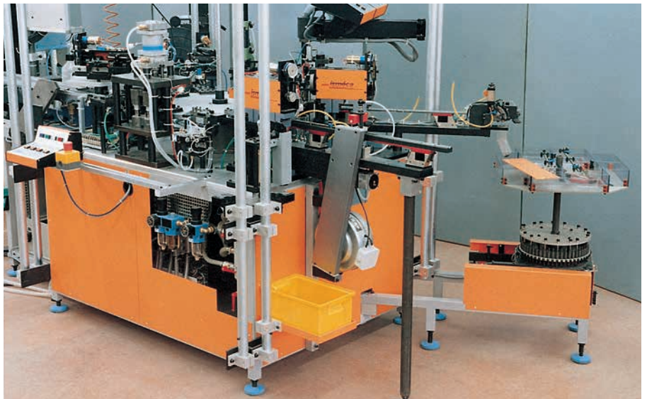
Protective covering guide device on automatic assembly unit, with weight compensation in the aluminium tubes.
