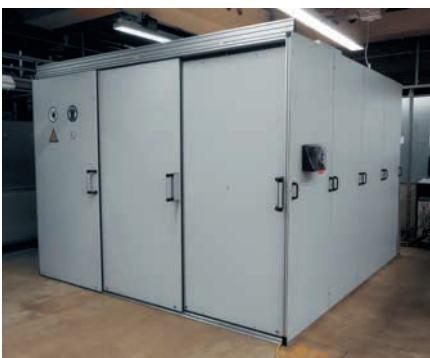
Noise protection cabin with 3-fold sliding door
