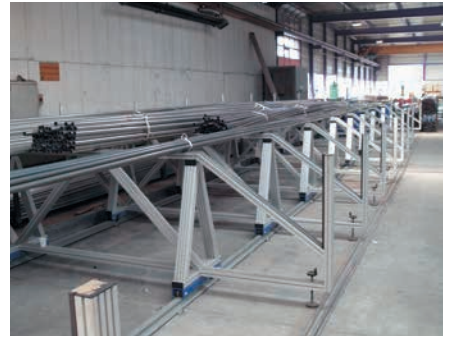
Long-item storage rack
