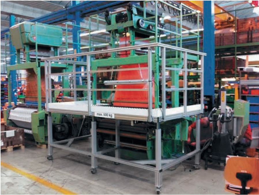
Lifting table as assembly aid around machine
