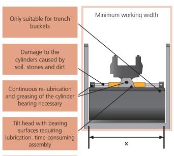
Over time. worn-out connection elements must be replaced
